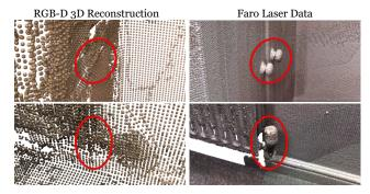
Figure 2. **Details in laser scans and RGB-D reconstructions.** Laser scans capture a higher level of detail, which is required for the geometrically fine-grained annotation of small interactive elements. In datasets with commodity-level RGB-D reconstructions (*e.g.*, ScanNet [11], MultiScan [46], Matterport [7]) these details are not visible.
